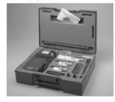
As compared with the F2000 carrying pouch, the K100 carrying case has additional room for three different three-phase current adapters, reel with measurement cable, telescoping rod, earth drills and 1081 probe.
