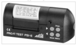
The PSI module is equipped with an RS232 interface, via which stored data can be transmitted at a later point in time to a PC, fully independently of the test instrument.
